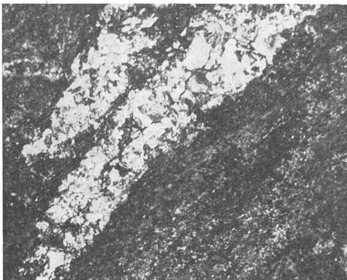
Fig. 6. In an aggregate polarizing rodingite mass elongated „miarolitic“ formations built by calcite, chlorite pyroxene. Danková, thin section, X pol., enlarged 45. x.
